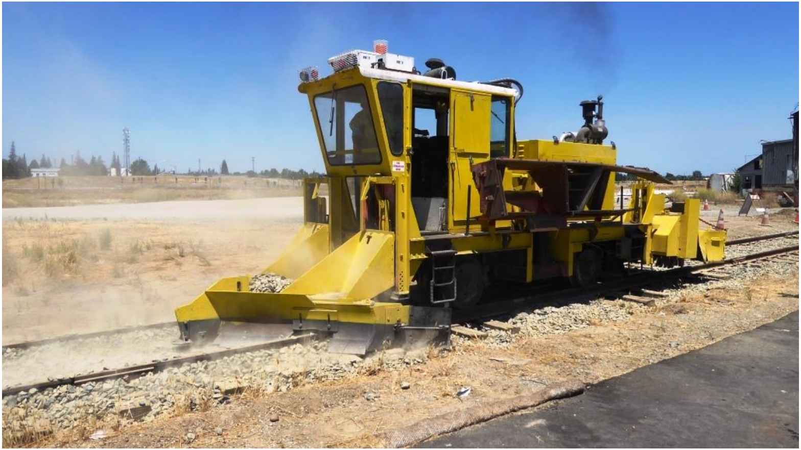
Rock gathers between the plows and is then spread evenly through the center of the track
