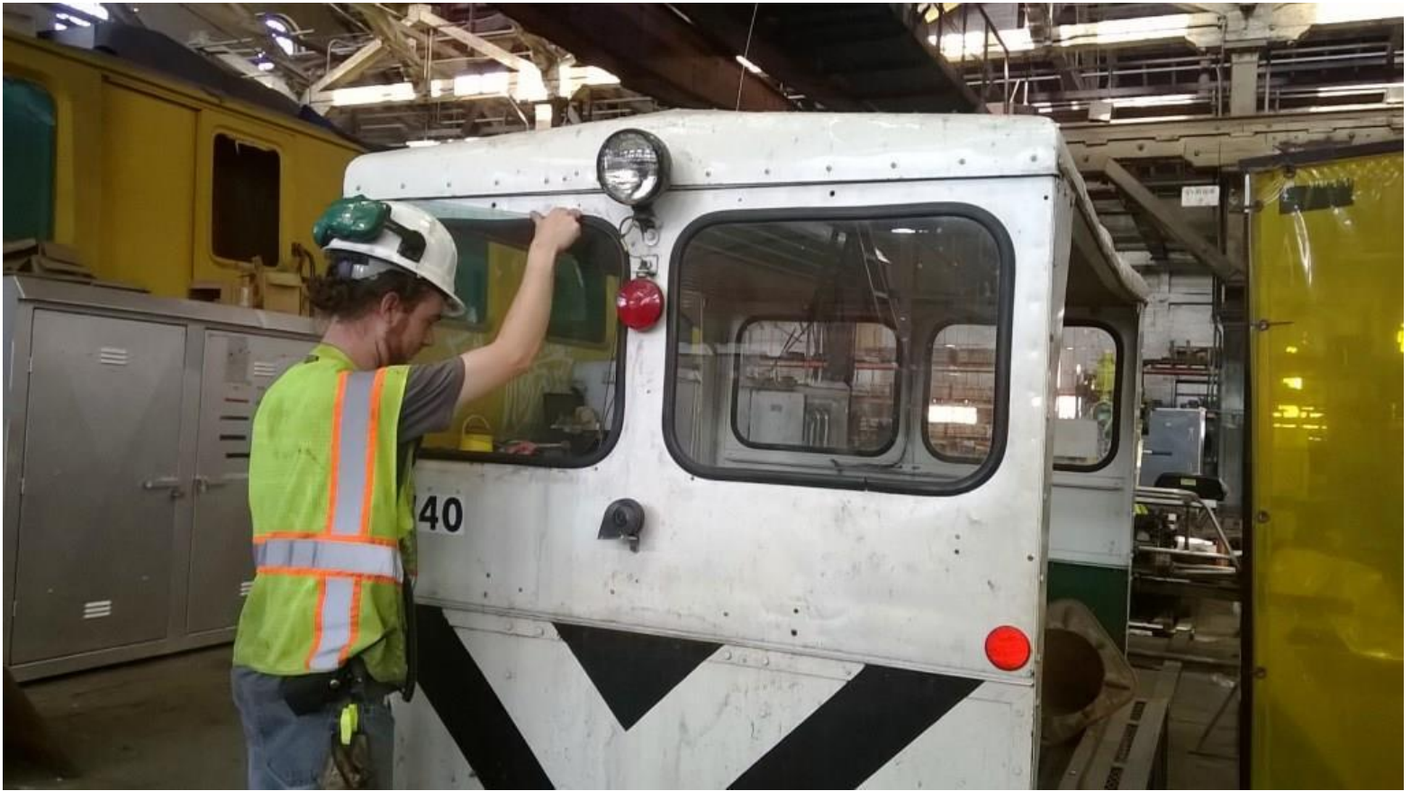
Matt installs a windshield on the A-4 motorcar
