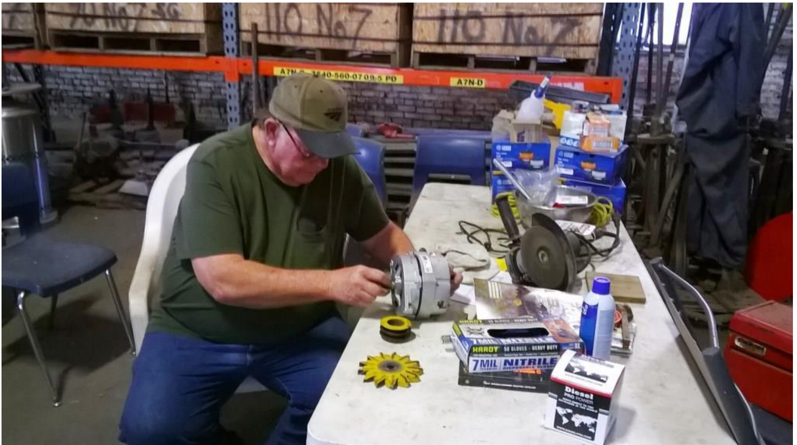
Gene does the necessary assembly work on the Jackson 125's new heftier alternator
